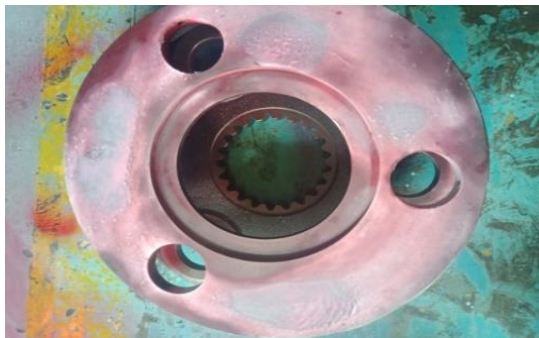
Gambar 3. Pengecekan Keretakan Carrier Assy
